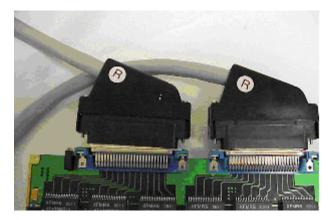
Figure D-1 Cable Attached to the ZXRTB24R
